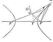
mer at G and G'. Draw F'G, cutting the curve in P Through P draw HPT, and it will be tangent to the hyper bola at P.
